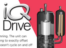
Inverter-driven rotary technology is different in that it is almost always running. The unit can modulate in five steps from 49 to 118 percent of capacity, instantly adjusting to exactly offset the cooling or heating demands on the home. Because the iQ Drive unit doesn't cycle on and off like a traditional system, it saves energy and considerably reduces sound levels. In fact, sound ratings are from 57-73 decibels depending on model – some of the lowest in the industry.
